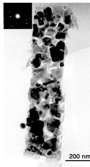
Figure 5. Electron micrograph of a V_2O_5 flake after heating at 600 °C, showing the formation of V_2O_3 nano-particles; the corresponding diffraction pattern is inserted.
